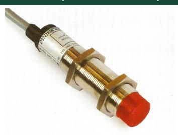
These Sensors are designed to provide better alternative to conventional limit Switches / micro switches. These are epoxy potted similar to other types of sensors to render IP67 protection and hence are suitable even in underwater applications. The load (AC Contactor / AC Relay / Solenoid Coil) is to be connected in series with the switch.
