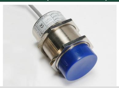
These Sensors are designed to work as solid state DC limit switches. The Sensors are connected directly in series with a load and have a bridge rectifier so they are not polarity conscious. The circuit is such that, when in off state, it allows very low current to flow through the load. However, a output load (such as relay) should be chosen, considering the voltage drop across the switch in the ON state. These sensors find wide application in electric control circuits and PLC's.
